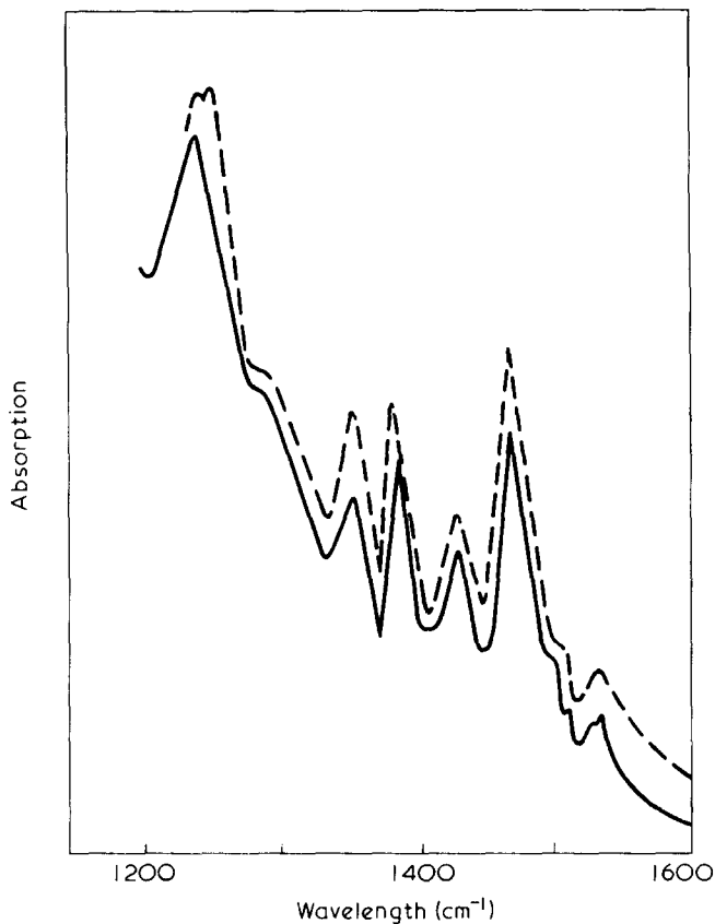
Figure 6 I.r. spectra of ultrafine POM fibrils in polarized light parallel (---) and perpendicular (—) to fibre axis
