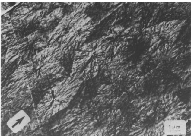
Figure 6 Electron micrograph of an ultramicrotomed section of IPS crystallized by swelling with dichloromethane vapour
